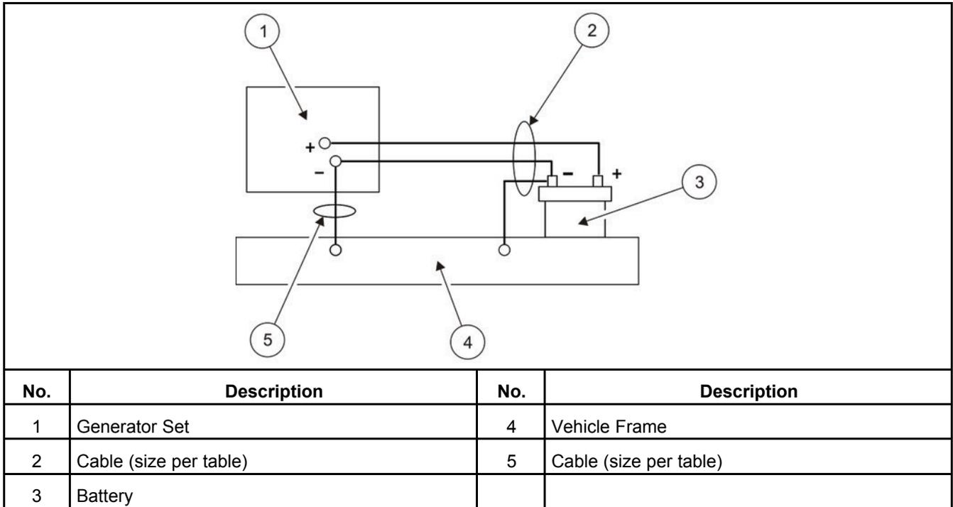
**FIGURE 13. FULL-LENGTH CABLE FROM BATTERY NEGATIVE (-) TERMINAL**
