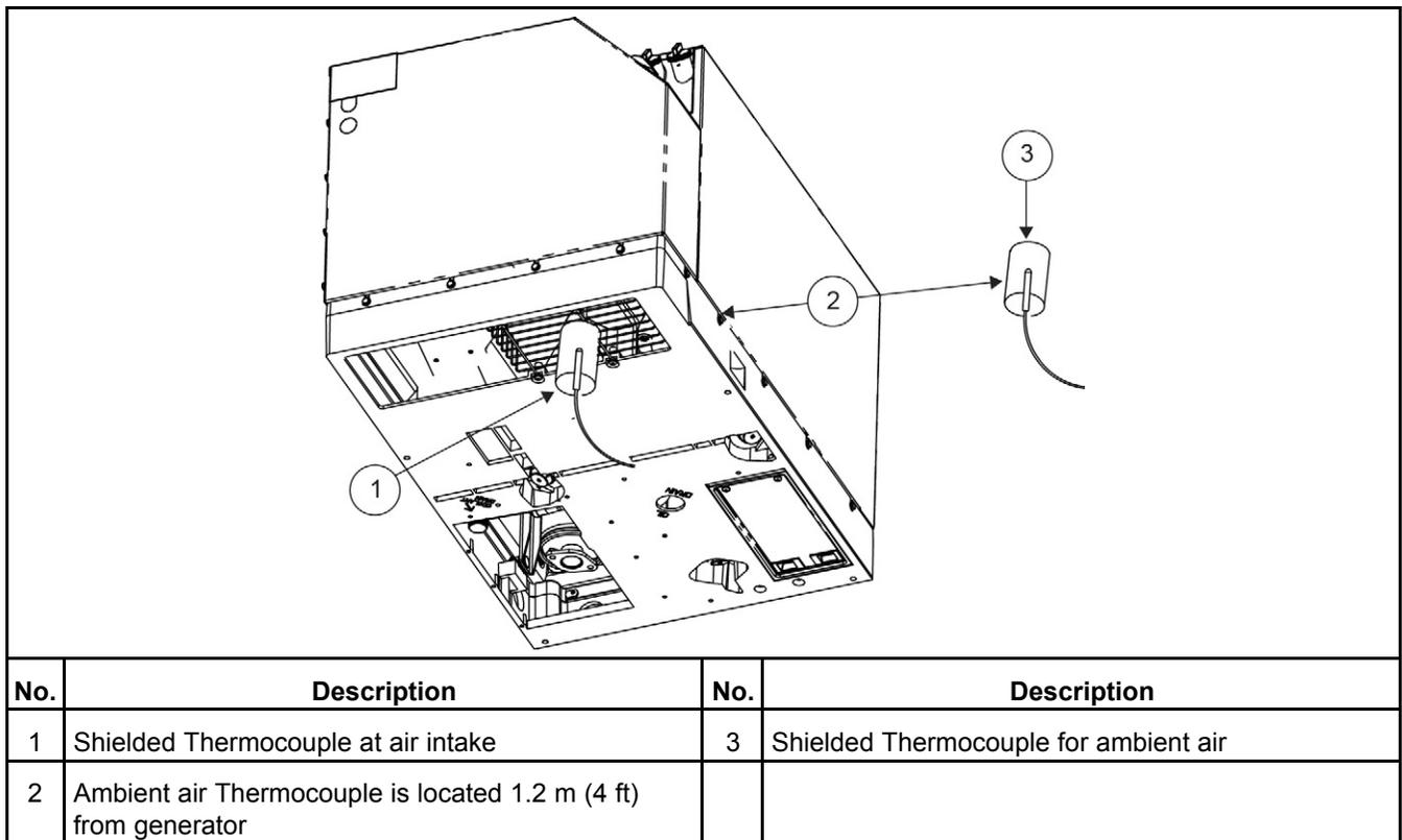
**FIGURE 16. THERMOCOUPLE LOCATIONS FOR HOT AIR RECIRCULATION TEST**
