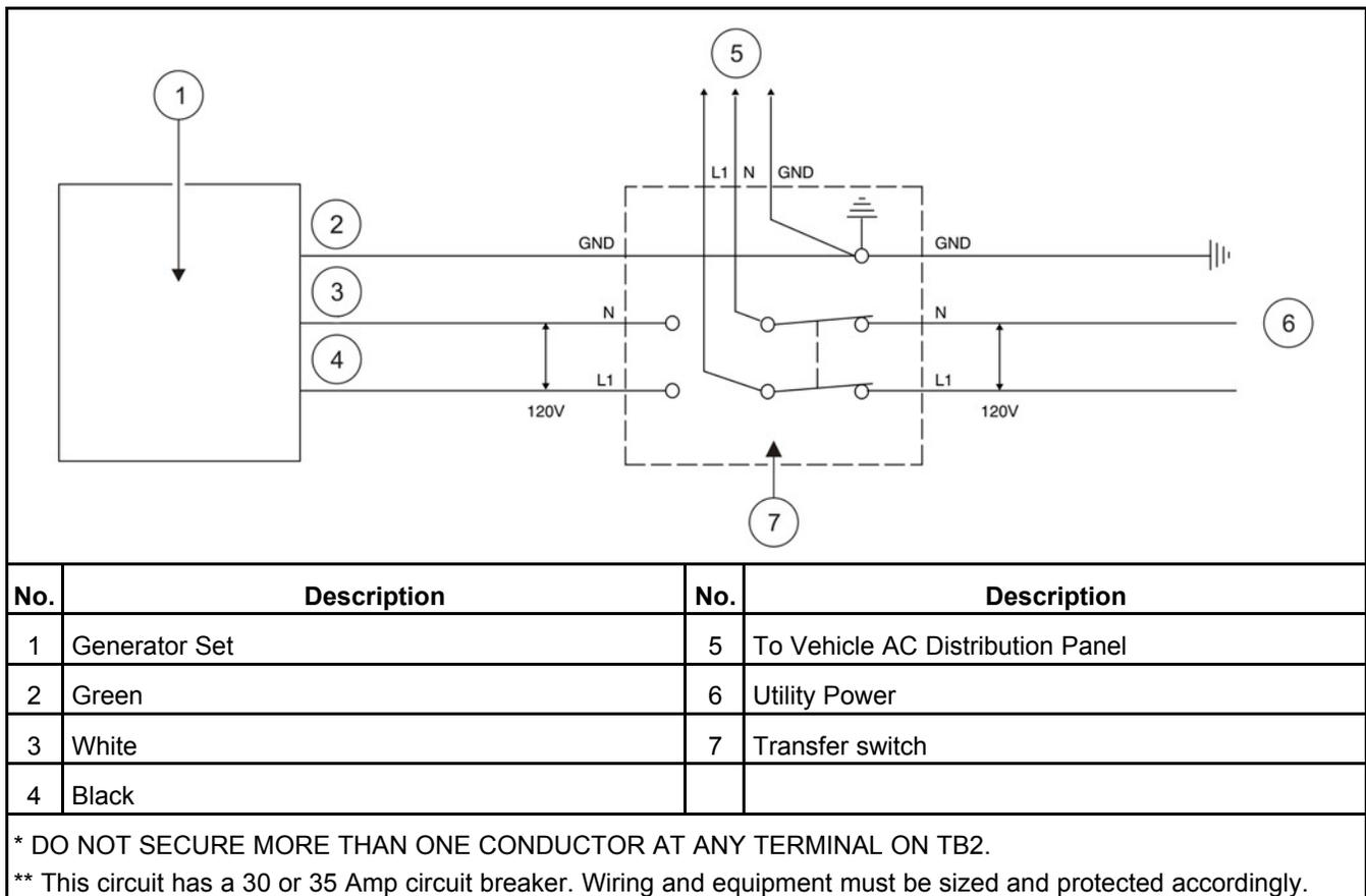
**FIGURE 10. TYPICAL CONNECTIONS WITH TRANSFER SWITCH AND UTILITY**
