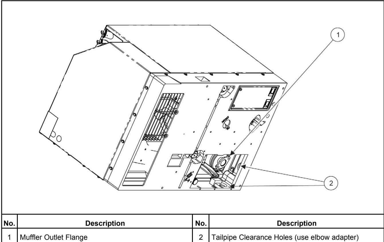
**FIGURE 3. TAILPIPE INSTALLATION**
