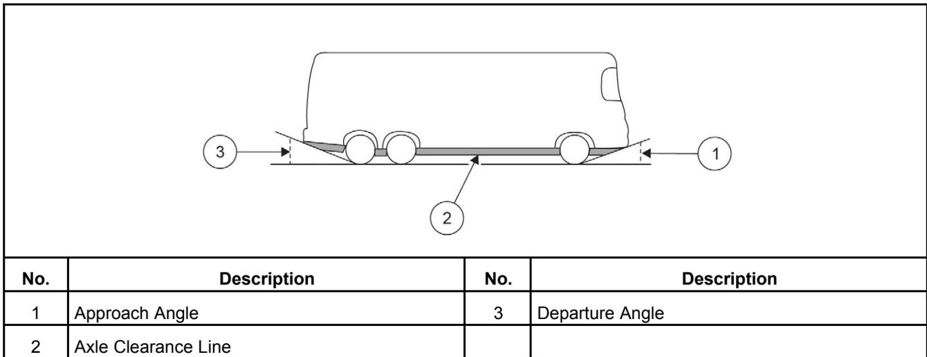
FIGURE 7. VEHICLE CLEARANCES - CLASS A RV
