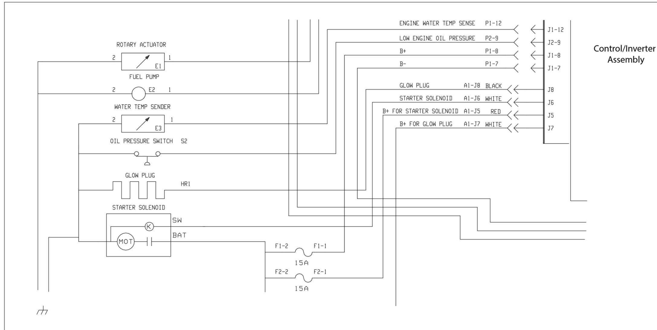
FIGURE 19. FC32 TROUBLESHOOTING WIRING DIAGRAM
