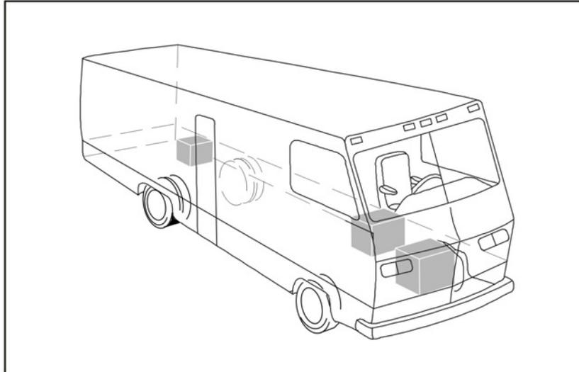
FIGURE 1. TYPICAL GENERATOR SET LOCATIONS - CLASS A RV
