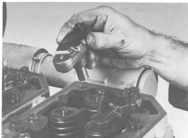
Install Jacobs exhaust valve crossheads, making sure that the adjusting screw locknut is loose and that the adjusting screw has been backed off and seated in its socket.
