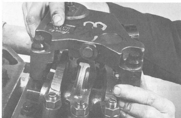
Carefully locate Engine Brake housing over rocker assembly.
