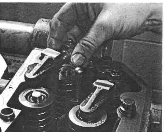
Remove Cummins exhaust valve crossheads.
