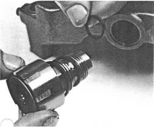
Lubricate the seal rings with engine lube oil before assembling. Install lower seal ring (1083) into the solenoid bore in the bottom of the housing. Install upper seal ring (1081) on the solenoid valve. Install center seal ring (1082) on the solenoid valve. Insert the solenoid with seals into the housing gently without disturbing the seal rings and turn all the way in.
