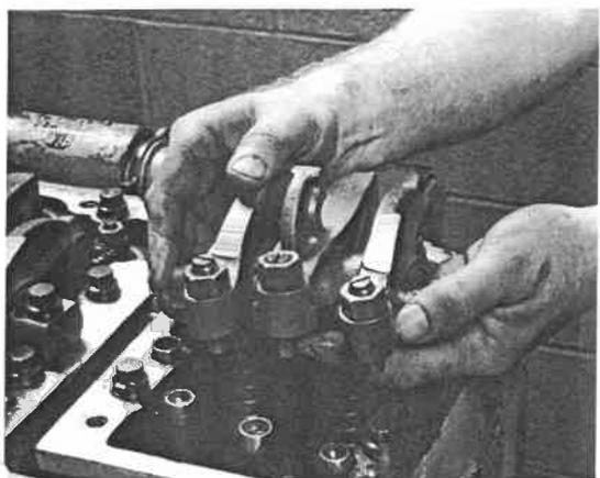
Remove rocker lever shaft holddown bolts and remove rocker shaft assemblies from the engine.
