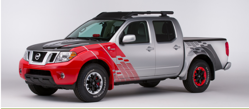
The Frontier Diesel Runners – Powered by Cummins. The truck has a 2.8L turbo diesel engine. Nissan and Cummins are evaluating the viability of the package.
