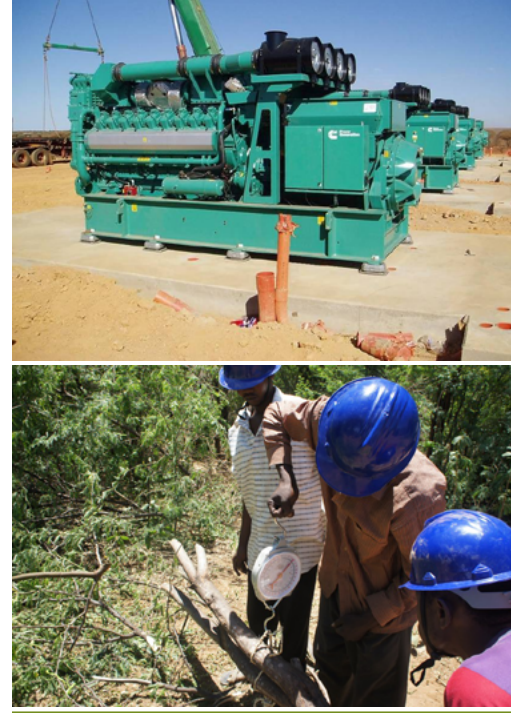
TOP Cummins’ QSV91 engine will produce electricity in Baringo, fueled by Juliflora , an invasive weed.
