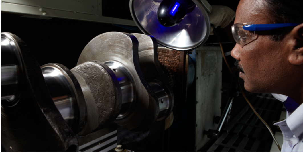
A Cummins employee uses ultrasonic inspection to verify that an engine crankshaft meets factory specifications.
