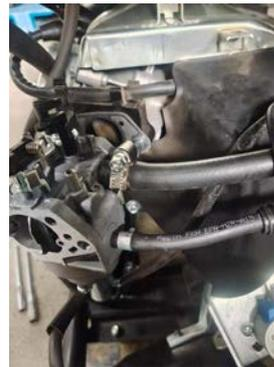
11. Remove the bolt on the bottom of the carburetor float.
