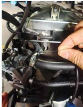
9. Remove the wire tie and wire clamp that fix the tube and wire harness.
