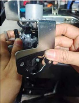
8. Remove the throttle lever and the spring C.
