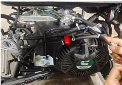
10. Remove the low pressure hose and the fuel hose by squeezing clamp and pulling off.
