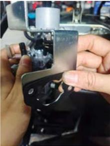
8. Remove the throttle lever and the spring C.
