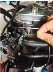
9. Remove the wire tie and wire clamp that fix the tube and wire harness.
