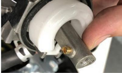
13. Reinstall float bowl gasket and then reinstall the float bowl. If the gasket is worn use the replacement included.
