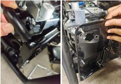
7. Remove the stepper motor assembly and the air gasket.
