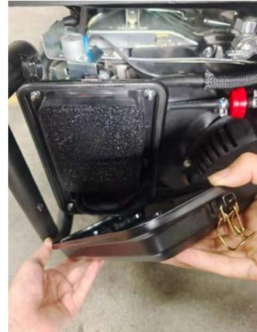
4. Remove the foam filter holder by removing the bolts.
