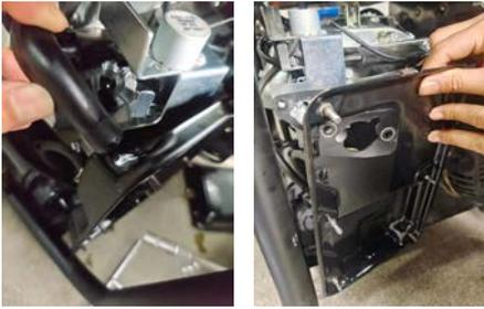
7. Remove the stepper motor assembly and air gasket.
