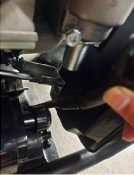
6. Pull out the breather tube from air filter assembly and then remove the air filter base.
