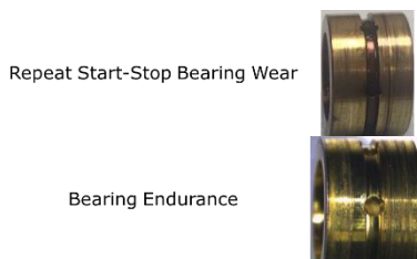
Figure 14: Turbine end journal bearing post turbocharger-based wear testing
