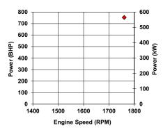
All data is based on the engine operating with a fuel system, water pump, lubricating oil pump, air cleaner, and alternator. The fan, optional equipment, and driven components are not included. Data is based on operation at SAE standard J1349 conditions of 300 ft. (91.4 m) altitude, 29.61 in. (752 mm) Hg dry barometer, and 77 °F (25 °C) intake air temperature, using No.2 diesel fuel only.
