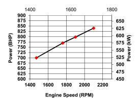
All data is based on the engine operating with a fuel system, water pump, lubricating oil pump, air cleaner, and alternator. The fan, optional equipment, and driven components are not included. Data is based on operation at SAE standard J1349 conditions of 300 ft. (91.4 m) altitude, 29.61 in. (752 mm) Hg dry barometer, and 77 °F (25 °C) intake air temperature, using No.2 diesel fuel only.
