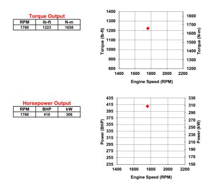
All data is based on the engine operating with a fuel system, water pump, lubricating oil pump, air cleaner, and alternator. The fan, optional equipment, and driven components are not included. Data is based on operation at SAE standard J1349 conditions of 300 ft. (91.4 m) altitude, 29.61 in. (752 mm) Hg dry barometer, and 77 °F (25 °C) intake air temperature, using No.2 diesel fuel only.
