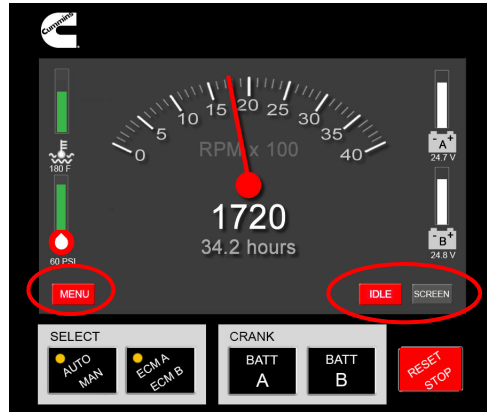
Figure 4-4 FPDP User Interface screen (electronic engine)
