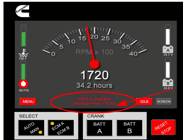
Figure 2-14 VSPLC inactive screen - red (sample)
