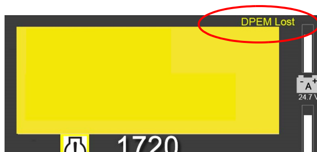
Figure 2-16 DPEM lost fault screen (sample)
