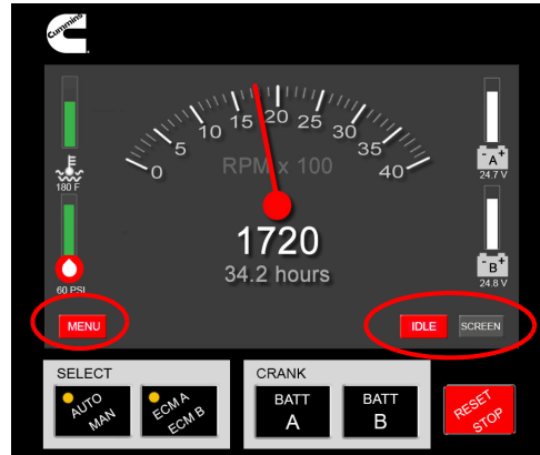
Figure 4-4 FPDP User Interface screen (electronic engine)
