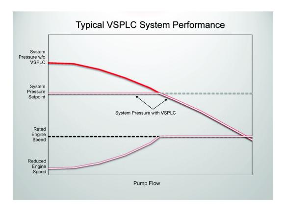
The CFP5E, 7E, 9E, 15E, and 23E models can be set at any specific pressure between 100 and 350 psi. The pressure must be set at the factory. All associated control loop parameters, including the pressure set point, are password protected such that they are not field adjustable. A Cummins Inc. representative must make and approve any changes to VSPLC settings.
