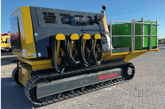
M5 tracked engine unit featuring Cummins X12
