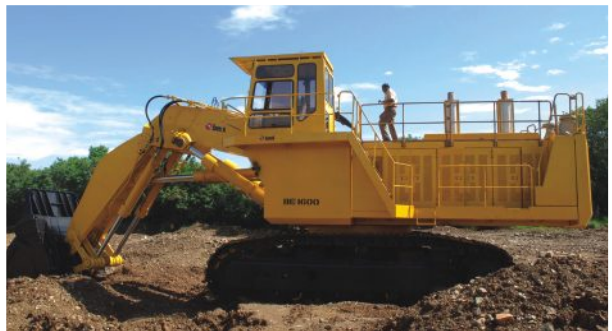
A power-packed solution The new electronic engine, QSX15 on BEML's 9.5m 3 (BE1600) Hydraulic Excavator
