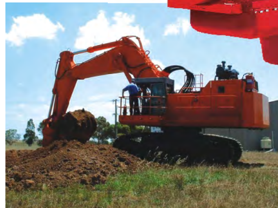
120T Excavator powered by Cummins QSK23.
