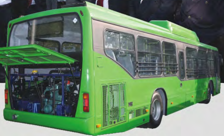
Delhi Transport Corporation's (DTC)'s latest environment-friendly bus supplied by Tata Motors powered by the Cummins B Gas International (BGI) engine.
