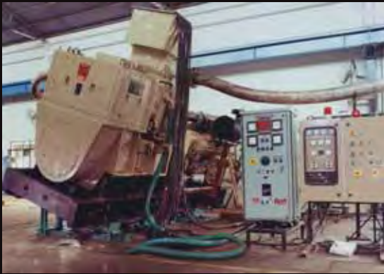
Indian Navy's Project "P-15A" - Cummins 1 MW DG set undergoing tilt test at Kothrud plant
