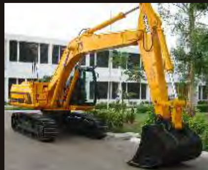
JS 200 Excavator with Cummins 6BT engine
