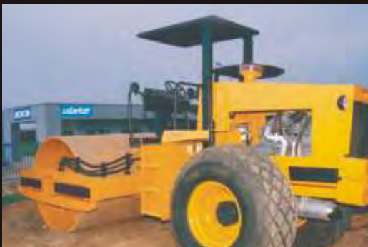
IR Compactor ISD 150 powered by 6BT
