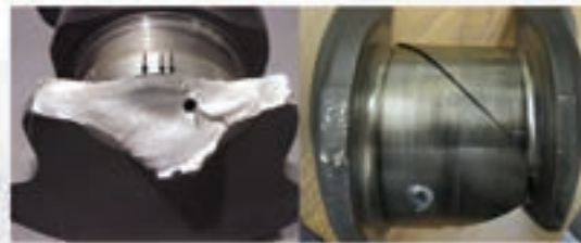
Bending fatigue failure
