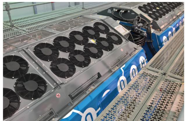
Multiple core fuel cell stacks are combined, sharing integrated cooling, ventilation and output regulation.
