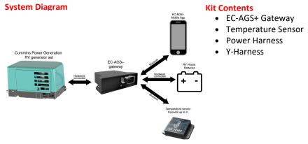
NOTE: Do not install EC-AGS+ Gateway directly in the RV generator set compartment.
