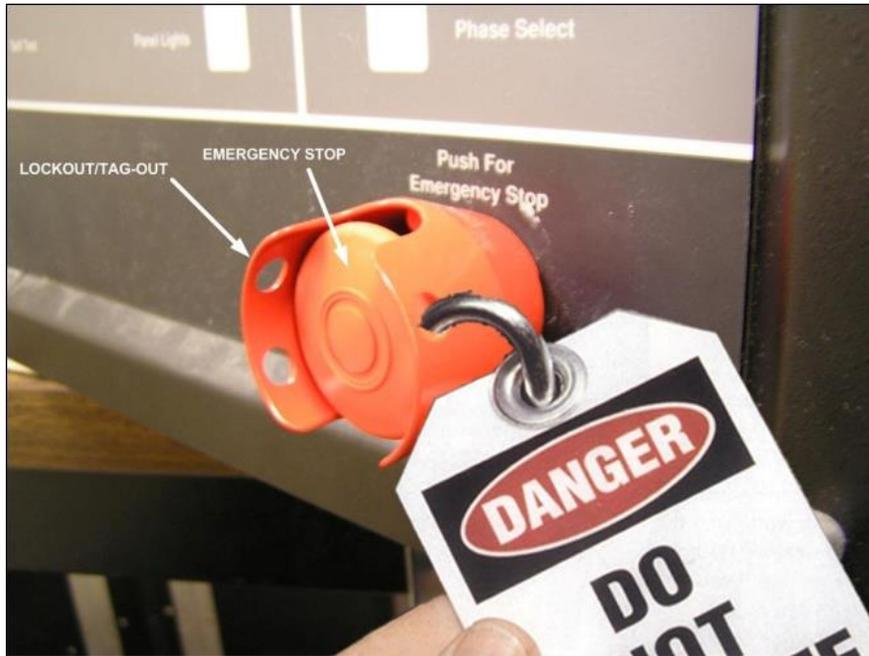
E-stop switch with lockable shroud
