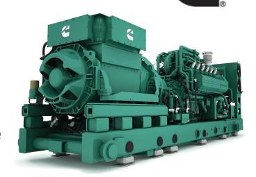
Alternator – Several alternator sizes offer selectable voltage and temperature rise with low reactance 2/3 pitch windings; low waveform distortion with non-linear loads, fault clearing short-circuit capability, class F or H insulation (see Alternator Data Sheet for details), bearing and stator RTDs and anti-condensation heater. Mechanically strengthened for use on utility paralleling with unreliable grid.
