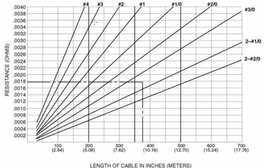
Resistance vs. length for various AWG cables sizes
