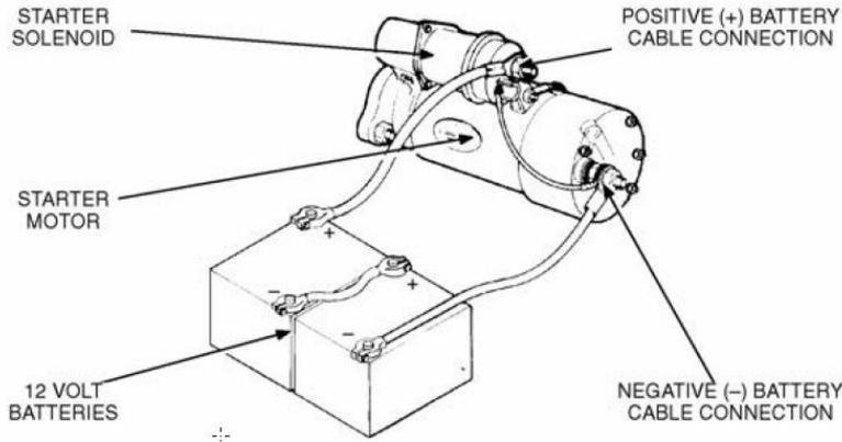
Typical electric starter motor connections
