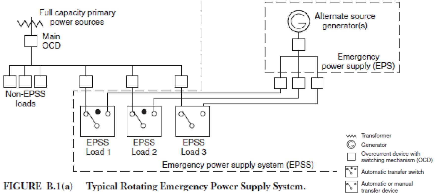
**FIGURE B.1(a) Typical Rotating Emergency Power Supply System.**
